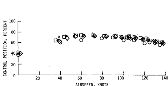
Fig. 7 SH-2F directional pedal control positions.
